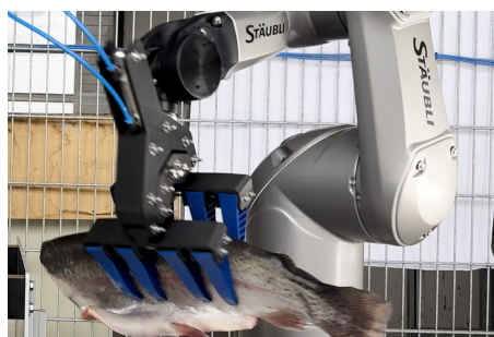
Figure 4: The manipulator is shown here grasping a fish. The grasping position is deliberately chosen; however, this goes beyond the scope of this work.
