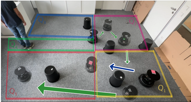
Figure 3: Scenario 2: R_c is instructed to move to Q_5 (red) from Q_3 (blue), but the shortest path through Q_4 (green) is blocked by a human. Hence it instead opts for an alternative route passing through Q_2 and Q_1 after requesting R_e to leave.
