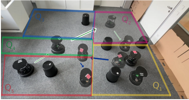
Figure 2: Scenario 1: R_c is instructed to go to Q_1 (yellow) from Q_5 (red), but has to go to Q_2 (purple) instead to request R_e (marked with a red flag) to leave.
