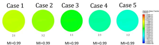
**Fig 9.** Mass fraction contour plots for different velocity ratios.
