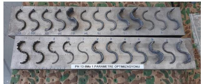
**Fig 3.** S shaped deposits of PH 13-8 Mo Stainless steel on 1050 Stainless steel substrate.
