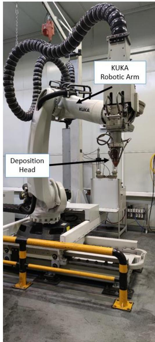
**Fig 1.** Robotic LMD system with co-axial powder nozzle and the accessories.
