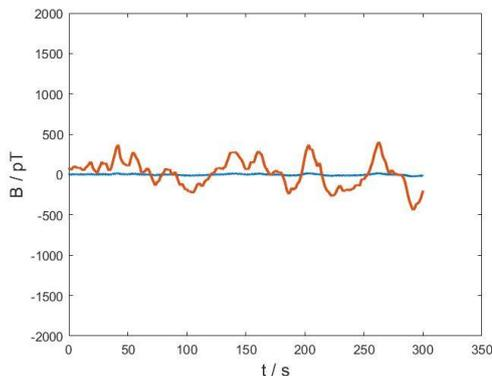
Figure 2: (a) OPM signals with PID control off. Both OPMs see the same background field fluctuations due to weak shielding of a two layer magnetically shielded room in the mHz range. At  $t=70$  s saturation occurs. (b) PID control activated reduces the fluctuations below 500 pT even for the OPM at the center of the coil (orange trace). The OPM used as input for the PID shows a far superior reduction as expected (blue trace).
