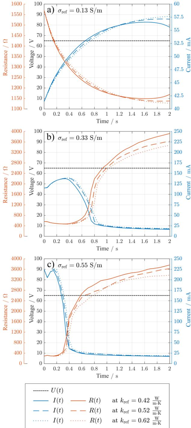
Figure 1: Simulation results of global current  $I(t)$  and tissue resistance  $R(t)$  at a constant applied DC voltage  $U(t)$  of 65 V of a tissue coagulation with three different initial values of thermal conductivity at an initial electrical conductivity of a)  $\sigma_{\text{ref}} = 0.13$  S/m, b)  $\sigma_{\text{ref}} = 0.33$  S/m, and c)  $\sigma_{\text{ref}} = 0.55$  S/m.
