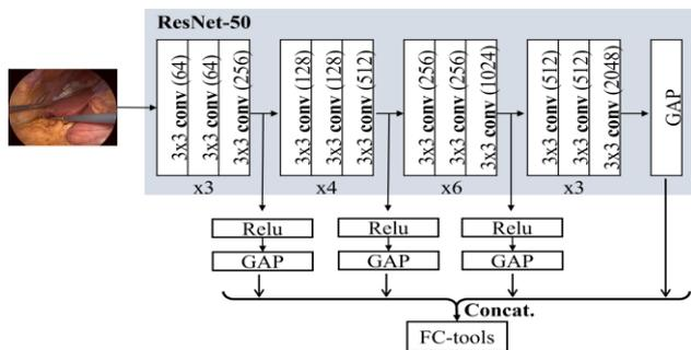
Figure 1: Proposed multi-layer fused feature (ResNet50-Fused).
