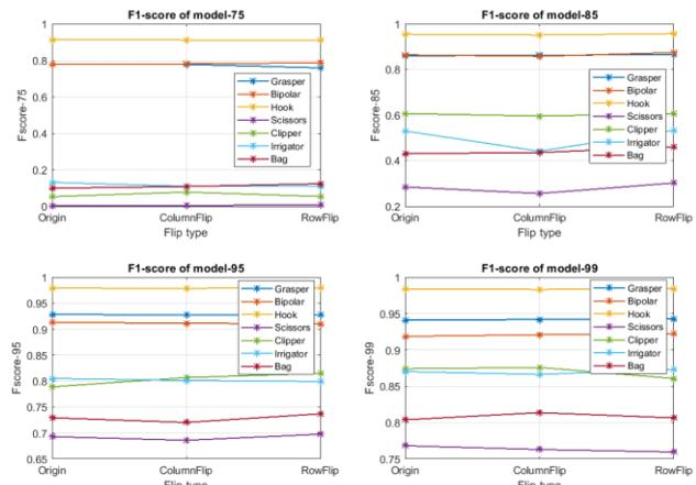
Figure 4: After additional training with image-flip, the F1-score of 7 medical tools on the original test set, the column-wise flipped test set, and the row-wise flipped test set.
