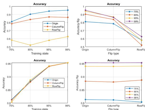
Figure 3: The 1st row showing the classification performance of four models on the original test set, the column-wise flipped test set, and the row-wise flipped test set. The 2nd row showing the classification performance of four models trained with additional pre-processing images on original test set, column-wise flipped test set, and row-wise flipped test set.
