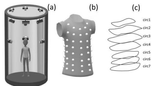
Figure 1: Sketch of the MoCap System (a) and the used compression shirt with MoCap markers (b). In (c) the circumferences are illustrated (based on the data of subject 1).
