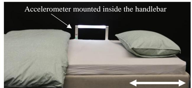
Figure 1: The Somnomat Casa applies translational vestibular stimulation in longitudinal direction. The attached handle has an integrated accelerometer to detect movement on the bed.
