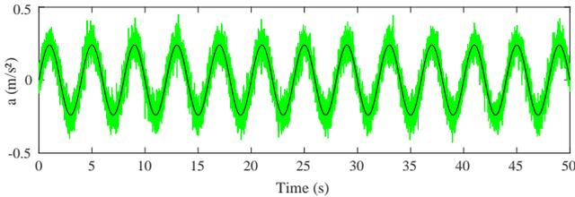
Figure 2: Black shows the desired- and green the actual noisy accelerometer readings. The variance  $\sigma^2$  reflects the noise of the accelerometer.
