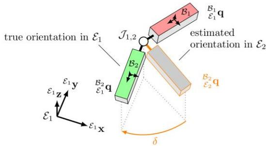
Figure 2: Heading offset of the orientation estimation of two connected bodies when using no magnetometer
