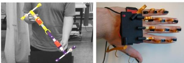
Figure 3: Experimental setups. Left: Mechanical test object. Right: Hand sensor system
