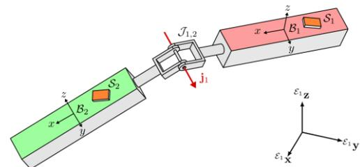
Figure 1: Mechanical model for a one-dimensional joint
