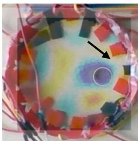
Figure 1: Superimposed image of an tdEIT image on petri dish with the white circle drawn to depict the cavity.
