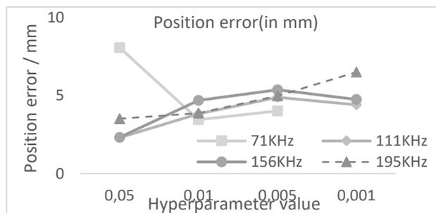
Figure 3: Position Error of tdEIT images when compared with actual cavity position for different hyperparameter values and frequencies.
