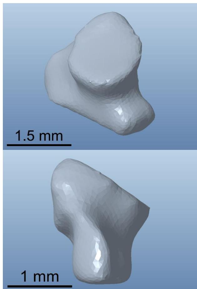
Figure 2: Top: Perspective view of digital model (STL-format) of patient-individualized RWN implant prototype. Bottom: Side view of digital model of implant prototype with build angles
