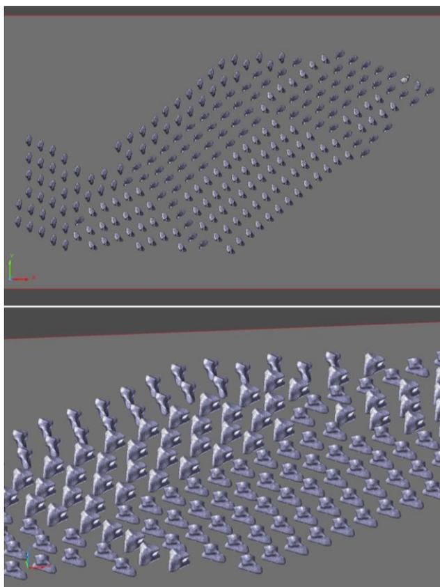
*Figure 3: Preparation of DLP-3D-printing. Top: The positioning of  $n = 250$  RWN implant prototypes on the digital build platform (top view). Bottom: Detailed view of RWN implant prototypes on digital build platform. Positioning of prototypes without any supporting structures (perspective view).*
