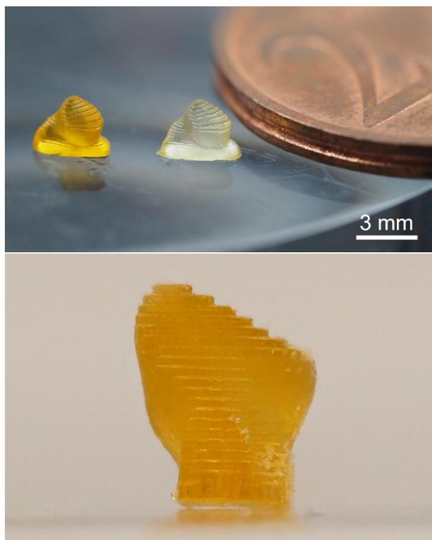
Figure 5: Top: DLP 3D printed RWN implant prototype manufactured without a post-curing process (left) and manufactured with a post-curing process ( $t = 30$  mins, right). The stain Orange G is faded as a result of the post-curing because of prolonged UV light exposure. Bottom: Side view of DLP 3D printed RWN implant prototype. There is staircase effect (3D print with layer height  $z_{\text{layer}} = 100 \mu\text{m}$ ).
