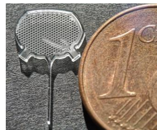
Figure 1: Fused silica mMS compared in size to Euro cent coin.
