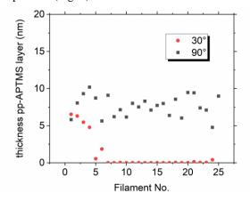
Figure 5: Thickness of the pp-APTMS layers as a function of the filament number for different plasma jet angles
