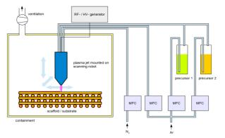
Figure 1: Used deposition setup with a plasma jet mounted on a scanning robot
