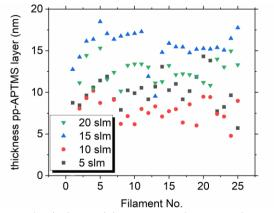
Figure 3: Thickness of the pp-APTMS layers as a function of the filament number of the scaffold structure
