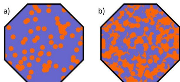
Figure 1: a) Mori-Tanaka scheme with orange inclusions embedded in a blue matrix. b) Self-consistent scheme with overlapping blue and orange phases.
