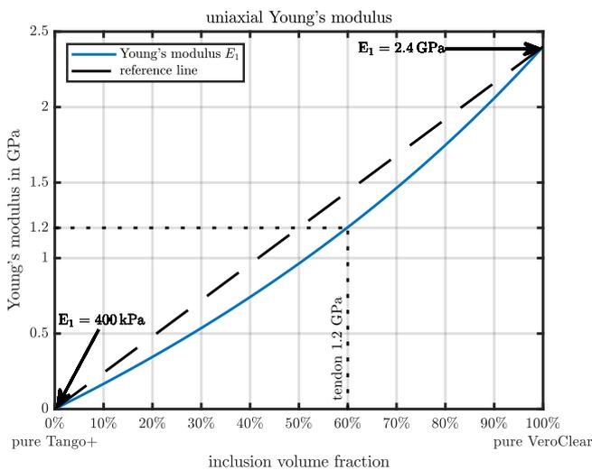
Figure 2: Uniaxial Young's modulus  $E_1$  from Tango+, VeroClear and the mixable bi-materials from these. A material mixture of about 60% VeroClear will show a Young's modulus of  $E_1=1.2$  GPa, corresponding to a human tendon as reported in ref. [19]. The reference dashed line shows a linear interpolation between the pure materials Young's moduli.
