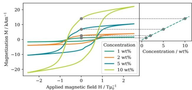
Figure 3: VSM measurements of the 3 mm cubes in different printed concentrations. A wide, hard-magnetic, hysteresis curve and a linear relationship between concentration and remanent magnetization is visible.
