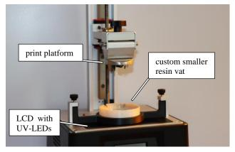
Figure 1: Printing setup with the modified resin vat and a finished print on the modified print platform.
