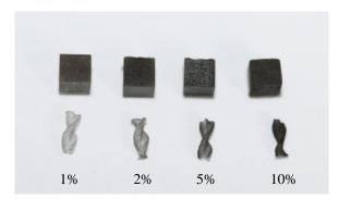
Figure 2: Printed 3 mm cubes and swimmers of 3 mm length [2] with different concentrations of NdFeB particles mixed in.
