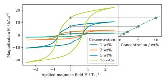
Figure 3: VSM measurements of the 3 mm cubes in different printed concentrations. A wide, hard-magnetic, hysteresis curve and a linear relationship between concentration and remanent magnetization is visible.
