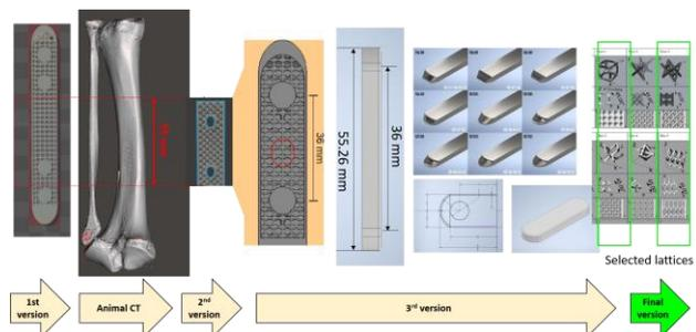
Figure 1: Demonstration of the prototype refining process.
