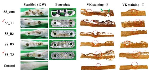
Fig. 5: The osteointegration of the examined 3D printed stainless steel 316L fixation plates. Left side: The regenerated bones and fixation plates showing ingrown tissue; Right side: Longitudinal histologic section with former bone defect geometry (red circle) and regenerated bone material within and above the defect location.
