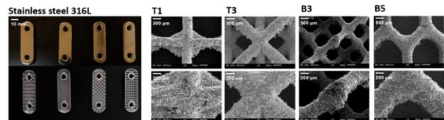
Figure 2: The printed bone plates and SEM images of the internal lattices.
