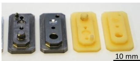
Figure 2: Milled steel mold (left) and DLP printed mold (right)
