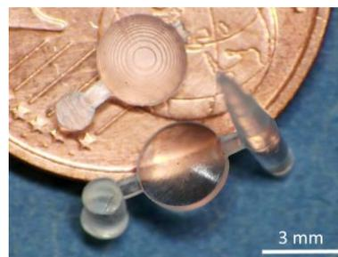
Figure 3: Top: Chip from  $\mu$ IM using DLP 3D printed mold. Surface shows staircase-effect. Bottom: Chip from  $\mu$ IM using milled steel mold. No staircase-effect, smoother surface.
