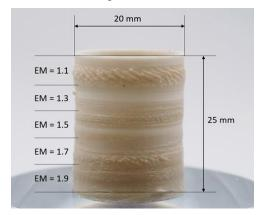
Figure 1: 3D printed EM tower for the detection of the optimized EM.
