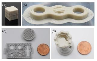
Figure 2: (a) Printed cube for density measurement; (b) Osteosynthesis plate with (23x7.5x2.5) mm in size; (c) Porous structures with 50% infill; (d) Benchmark part chess tower featuring fine internal details
