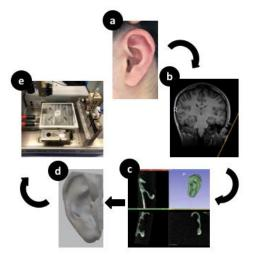
Figure 1: Workflow to produce three-dimensional ear model: (a) image of the unaffected left ear (b) magnetic resonance imaging of the unaffected ear; (c) 3D reconstruction; (d) mirroring of the ear; (e) 3D printing of the model
