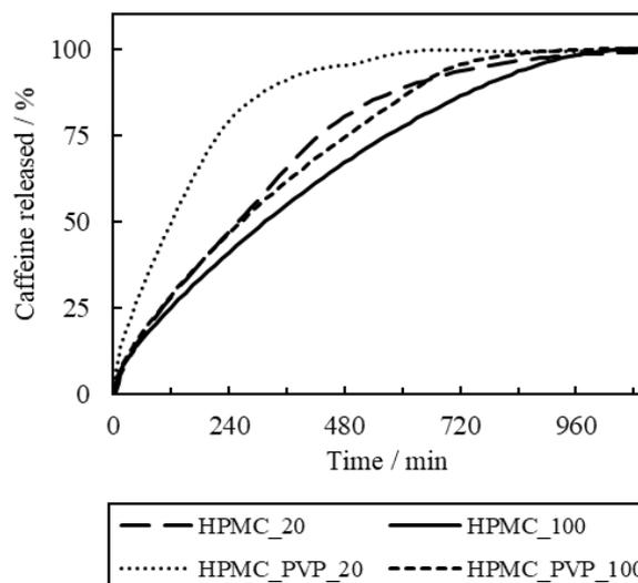
Figure 2: Drug release graphs of the different 3d printed batches with 20% and 100% infill and addition of PVP K12 (mean of  $n=6$ ).
