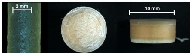
Figure 1: Reflected light images of the HPMC filament (left side) and the printed HPMC<sub>20</sub> tablets (middle - top view; right side - side view).
