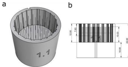
Figure 1: Cups with struts printed by point exposure with different laser powers and exposure times to determine the influence on the strut thickness. (a) schematic picture, (b) sketch with dimensions.
