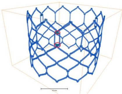
Figure 2. The reconstructed S3 type frame with pores.
