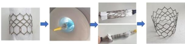
Figure 3. The deployment procedure of the S3 type frame.
