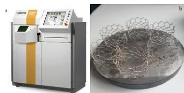
Figure 1: (a) SISMA MySint 100 printer, (b) S3 type frames on the metal plate.
