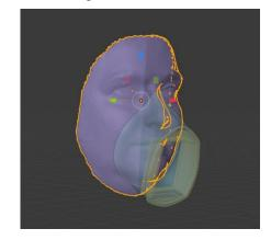
Figure 2: Integration between facial scan and "MyFaceMask" add-on on Blender to produce tailor-made 3D printed filtering masks.
