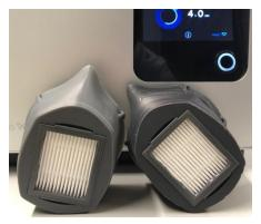
Figure 1: 3D printed masks with a Vat Polymerization printer and elastic resin.
