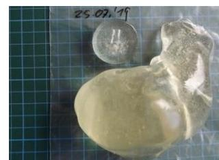
Figure 1: cast gelatine liver phantom sample in a 50% scale for evaluation and a reference measuring body.
