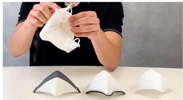
Figure 1: different development iterations of cirp's reusable respirator mask: pure SLS (right), SLS with soft sealing lip (mid right), 2-part IM (left) and 3-part IM solution (above).
