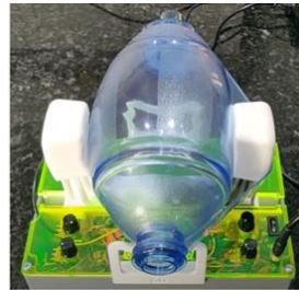
Figure 3: Resultant operational automated ventilator device.
