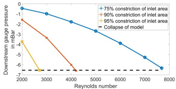
Figure 3: Downstream gauge pressure measurements for the determination of the critical closing pressure were carried out. The measurements were made with three varying constriction degrees of the inflow area. Flow was increased until the downstream pressure reached the critical closing pressure. A reduction of the inflow area leads to a decrease of downstream pressure. As soon as the downstream pressure falls below the critical closing pressure (dotted line) the model collapses.
