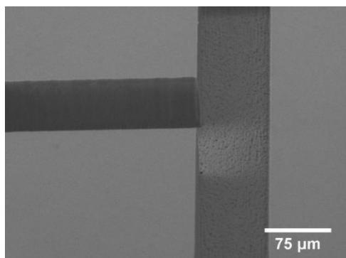
Figure 1: Example of SLE made microfluidical channel. Well-defined channel walls with minimal taper are evident. Surface roughness – less than 1  $\mu\text{m}$  RMS.
