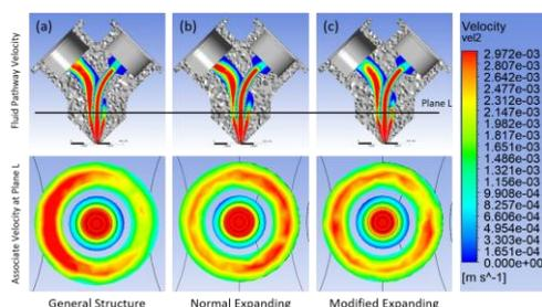
Figure 3: Fluid pathway and associated fluid velocity profiles for (a) compression co-axial nozzle without expanding chamber; (b) with a large expanding chamber nozzle; (c) with a small expanding chamber.
