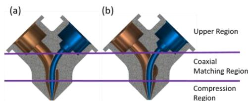
Figure 2: Schematic of co-axial nozzle (a) conventional co-axial nozzle; (b) novel expanding chamber nozzle.
