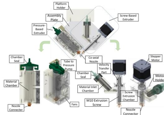
Figure 4: Co-axial extrusion printing head with one pressure-based and one screw-based extruders with temperature controlling system.
