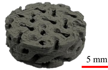
Figure 5: piston-based extruded Mg4.5Gd alloy, courtesy Fraunhofer IAPT
