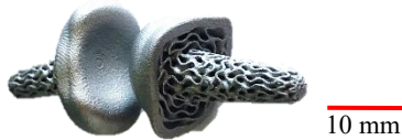
Figure 1: BJT-processed and polished finger joint implant for the proximal phalanx (left) and metacarpal bone (right), courtesy Fraunhofer IAPT
