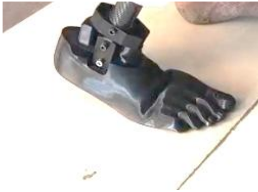
Figure 13: Shows the compliant bending of forefoot.
