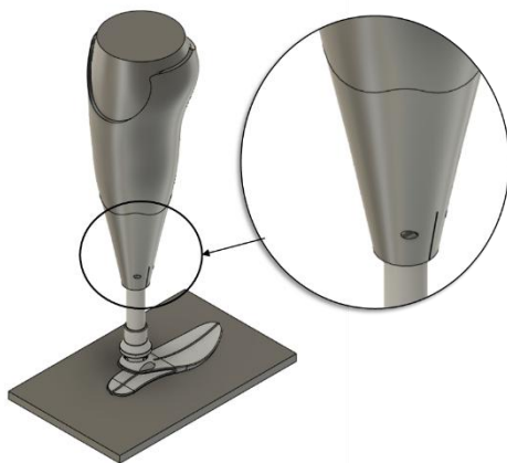
Figure 11: Shows the improved design of socket-pylon interface, designed considering additive manufacturing process.
