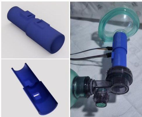
Figure 8: Orifice tube with embedded sensors for tidal volume calculation.
