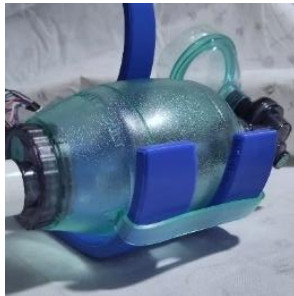
Figure 7: Optimised 3D-printed bracket for BVM.
