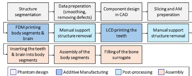
Figure 5: Simplified workflow used for the phantom.
