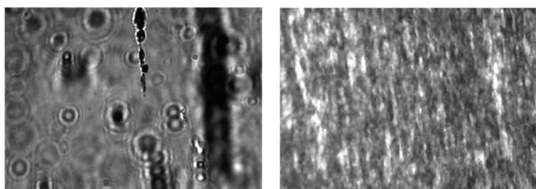
Figure 2: Light microscopy images ( $\times 63$  magnification) of SZ2080 with incorporated magnetic nanoparticles. The particles show a vertical alignment due to the applied magnetic field during baking. The in-house synthesized particles (left) and (II,III) iron oxide powder particles (right) were incorporated with 1 wt.% into the resin.
