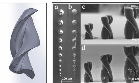
Figure 3: Left: CAD-model of the Savonius shaped object [8]. Right: 10 kV SEM micrographs of swimmers with (a,c) in-house and (b,d) commercially available iron oxide particles. Fabrication parameters: 780 nm, 15mW, 5000 $\mu$ m/s.
