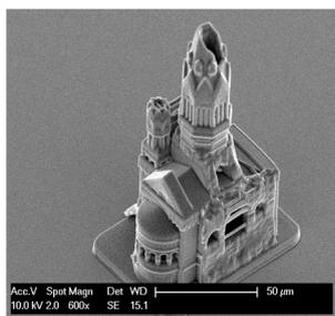
Figure 1: 10 kV SEM micrographs of Kaiser Wilhelm Memorial Church fabricated by multi-photon laser structuring.
