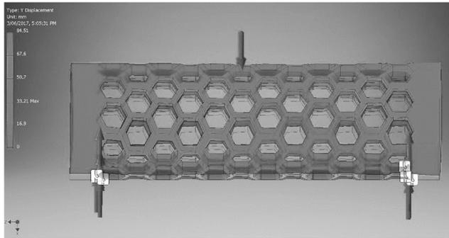
Figure 3: Simulated example of the load points for the mechanical testing of the samples.
