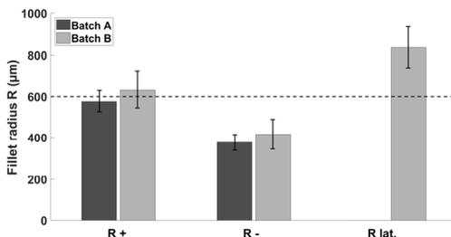
Figure 3. As-built fillet radius measured in batches A and B in the various locations of the lattice. “R+” and “R-” indicate the fillet radii measured in the plane normal to the printing plane, on the upper and on the lower side of the horizontal struts, respectively. “R lat” refers to the fillets measured in the printing plane. The dashed line indicates the as-designed value ( $600 \mu\text{m}$ ).
