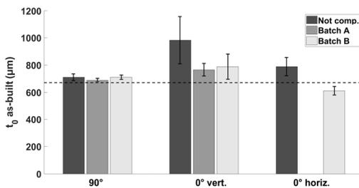
Figure 2. As-built strut section parameters of batch A and B with standard deviation classified according to their angle to the printing plane compared with the non-compensated specimens described in [3]. The dashed line indicates the as-designed value ( $670 \mu\text{m}$ ).
