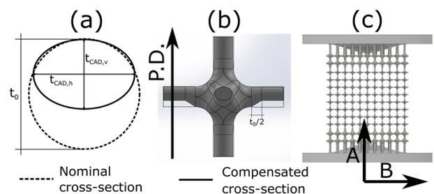
Figure 1. The compensation concept: (a) the CAD strut cross-section (defined by  $t_{CAD,h}$  and  $t_{CAD,v}$ ) is designed with the aid of the compensation model to produce the desired ( $t_0$ ) cross-section after manufacturing (horizontal struts); (b) compensated CAD of the unit cell (note the transition segment of length  $t_0/2$ ); (c) specimen for fatigue testing (the arrows indicate the printing direction for each batch).
