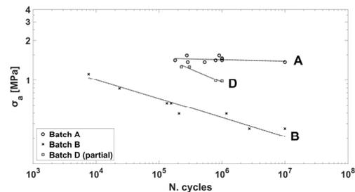
Figure 4. S-N curves measured from the fully reversed fatigue tests, for each batch of specimens. The dotted lines represent the linear regression of the experimental data.
